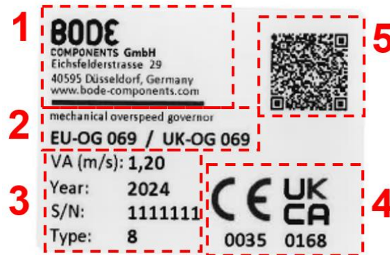
Figure 1: Example Type Label of an Overspeed Governor
